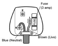
Class II Plug Wiring Diagram
