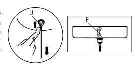
5. Support your fitting and connect the house wiring to the terminal block – see expanded wiring details below. NOTE: This is a Class II fitting and must NOT be earthed. Ensure no loose strands are left out of the connection block.
